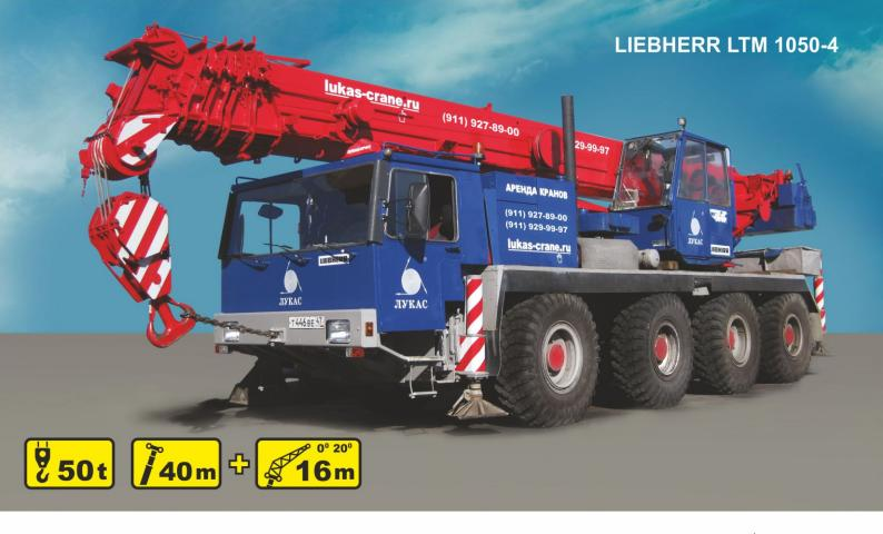
The LIEBHERR LTM 1050 - 4 mobile crane has a loading capacity of 50 tons, the main boom of 40 meters and the lattice jib of 16 meters.
